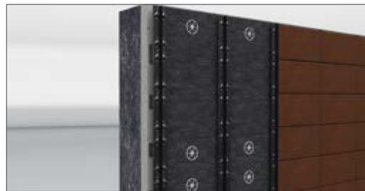
Mount the T-profile with approved fastening means
